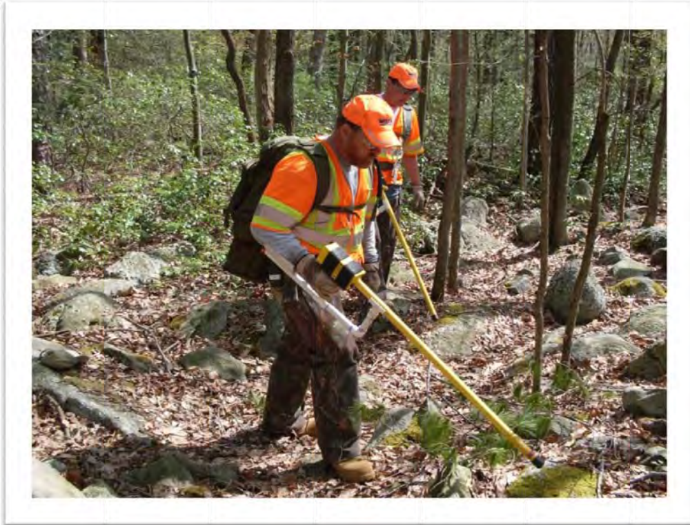
UXO Technicians performing Analog-Assisted Visual Survey in SGL211
