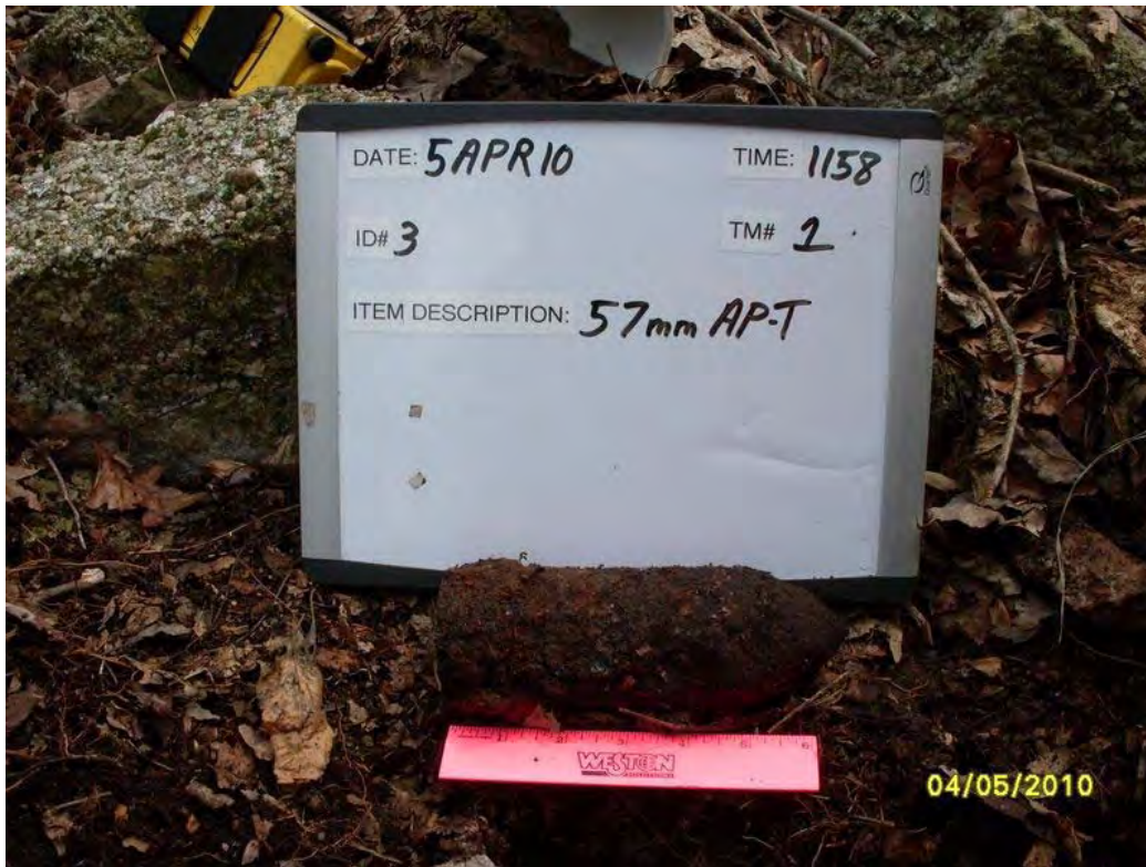
Munitions Debris: 57mm APT (solid & inert) excavated in SG211
