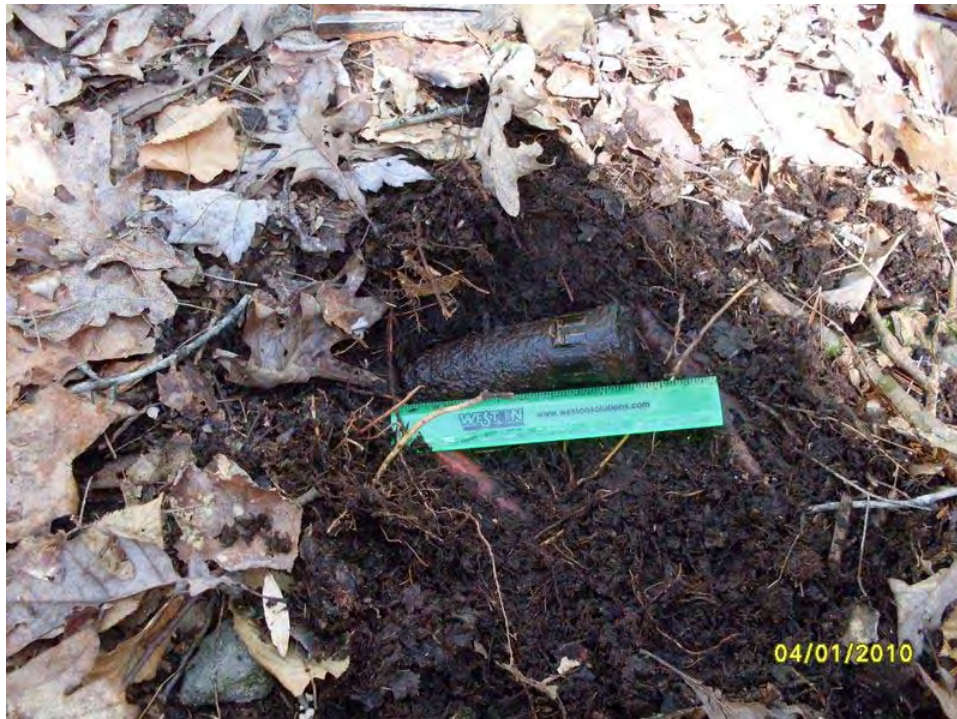
37mm APT (solid inert) excavated adjacent to Stony Creek
