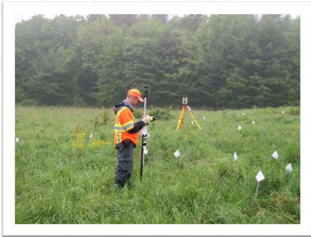
Field Technician reacquiring anomalies in DGM grid DI402 in Area E in SGL211
