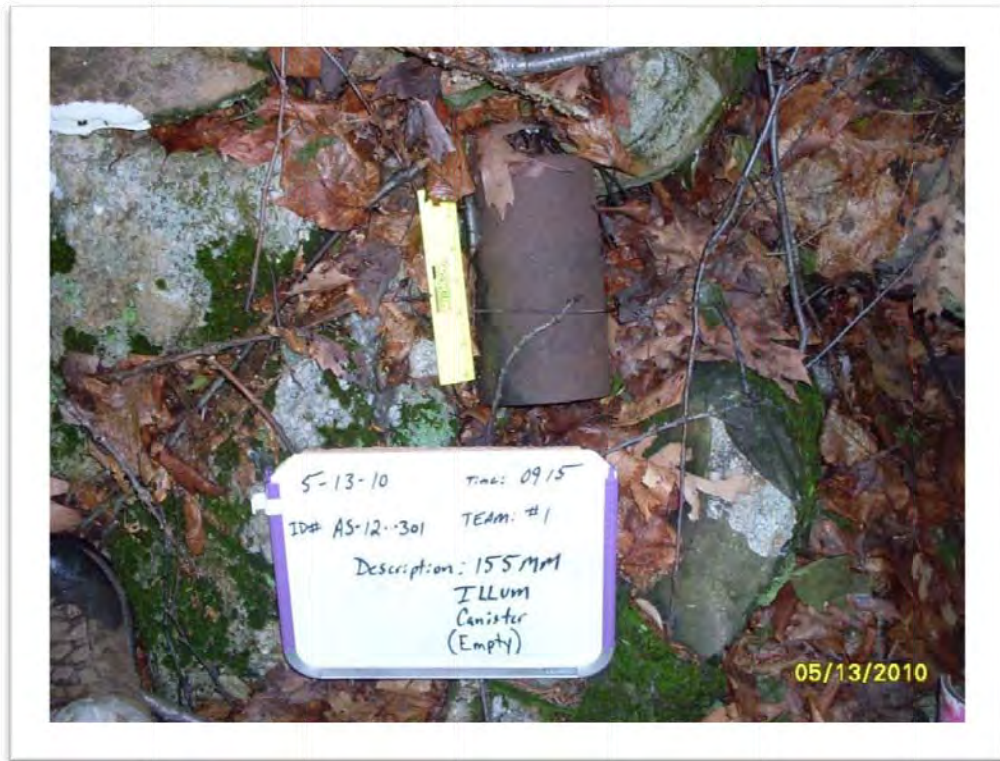
Munitions Debris: 155mm Illumination Canister (empty) recovered in SGL211.
