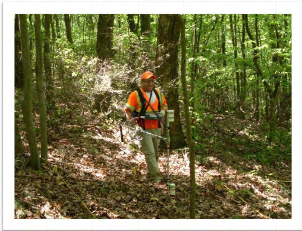
Geophysical Technician collecting data in a DGM grid in SGL211
