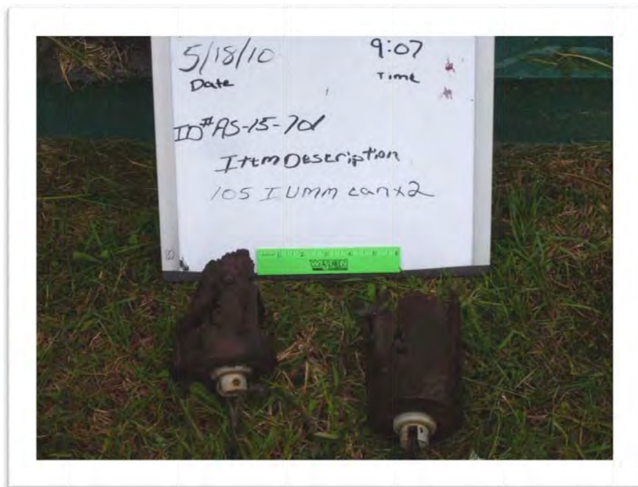
Munitions Debris: 105mm Illumination Canisters (empty) recovered from SGL211.
