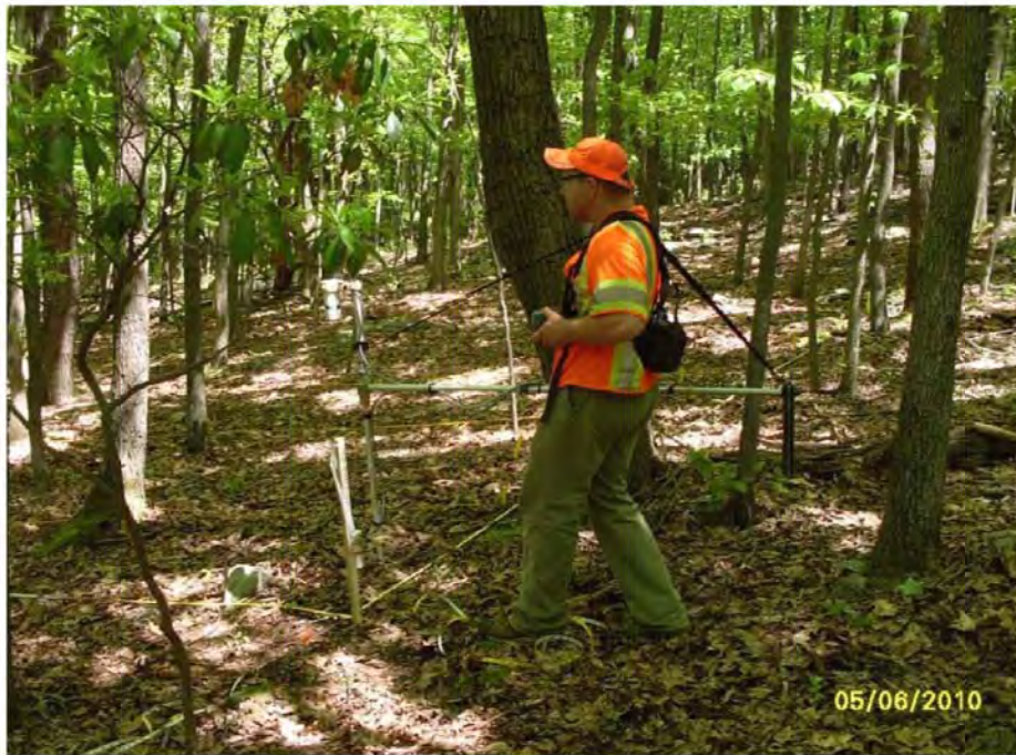
Geophysical Technician collecting data in a DGM grid in SGL211
