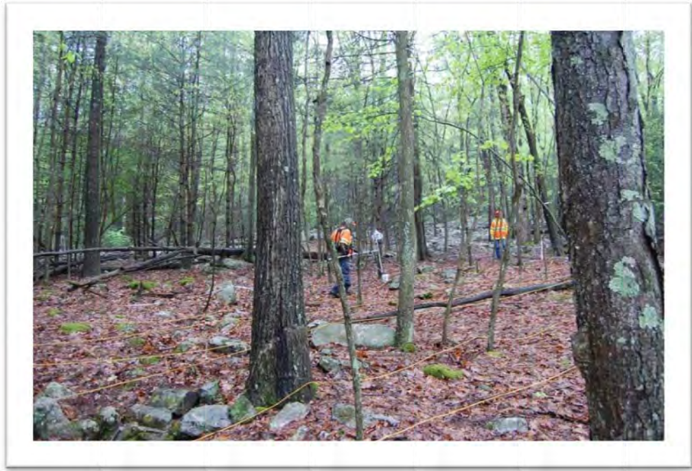
Geophysical Technician collecting data with the G-858 Magnetometer in grid C1A4-01
