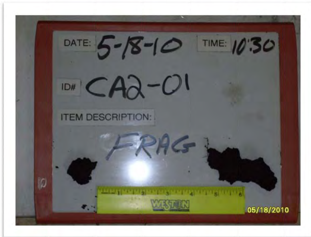
Munitions Debris: Frag recovered from DGM grid CA2-01 in SGL211.
