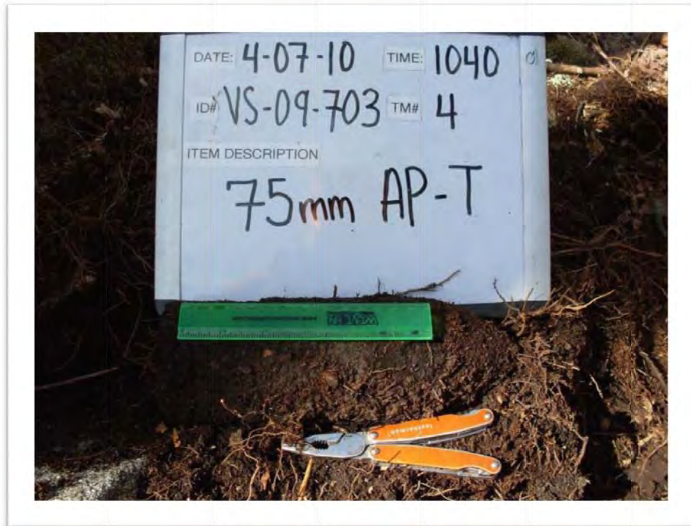
Munitions Debris: 75mm APT (solid & inert) excavated in SG211
