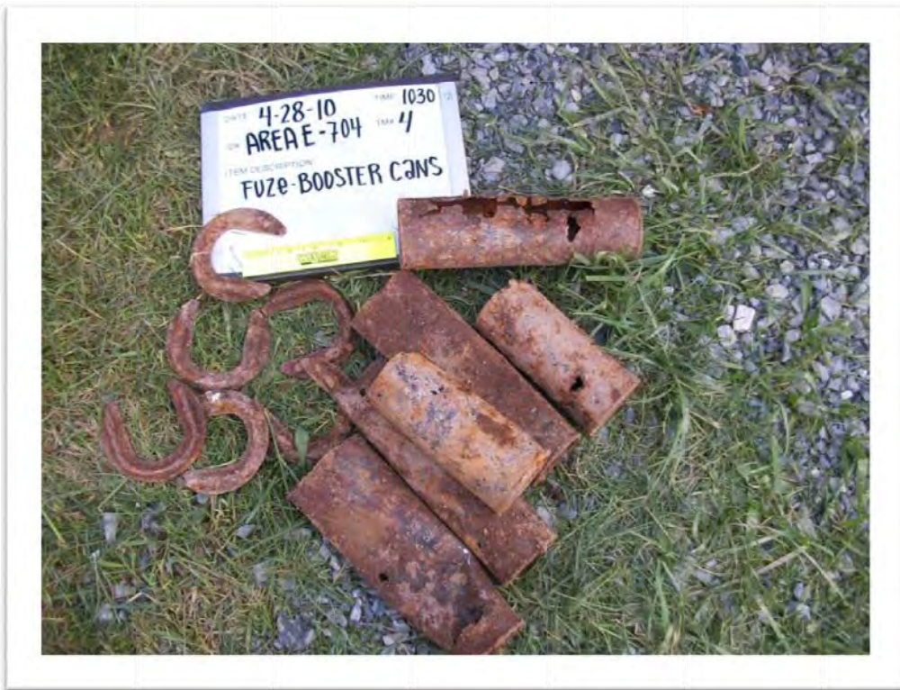
Fuze booster shipping containers excavated in Area E
