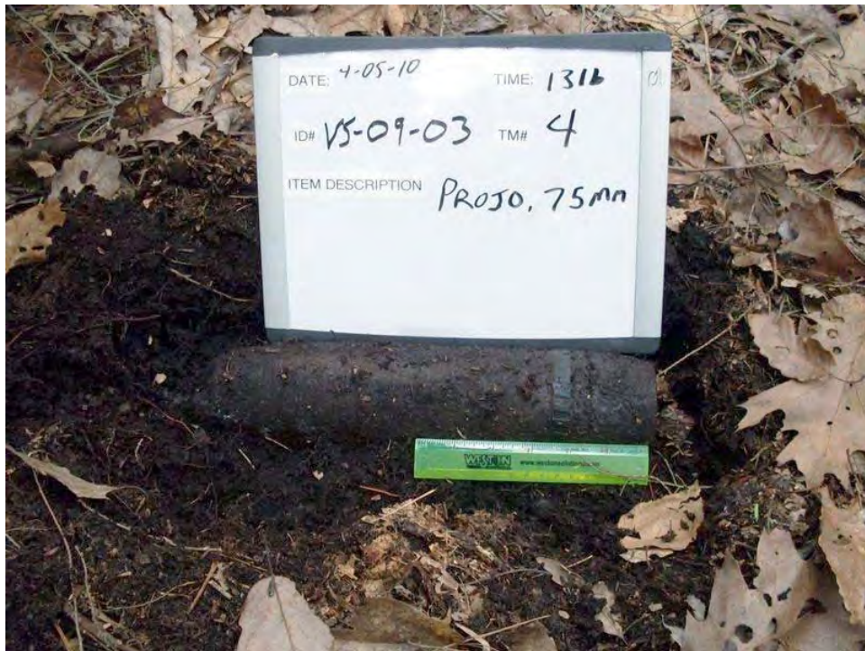
UXO Item: 75mm HE projectile excavated in SG211
