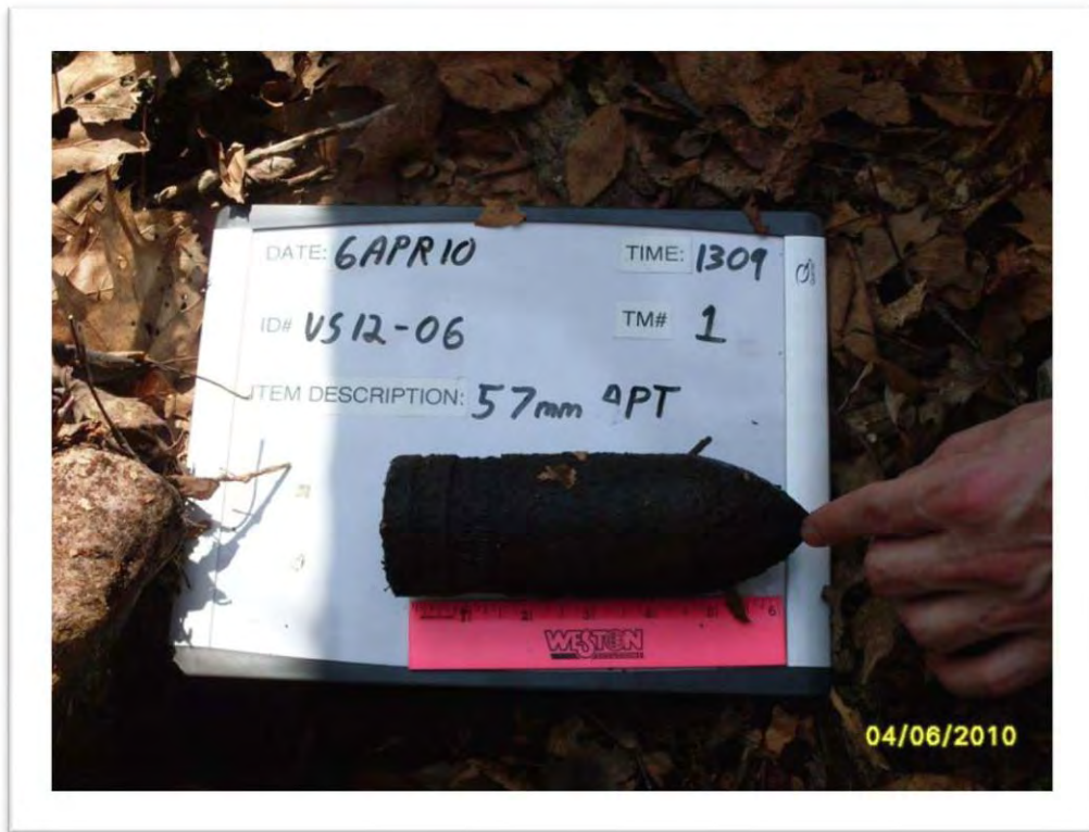
Munitions Debris: 57mm APT (solid & inert) excavated in SG211
