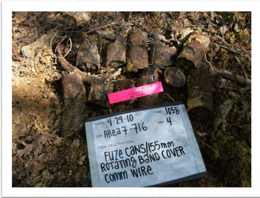
Fuze shipping containers, 155mm rotating band covers, and comm wire excavated in Area E
