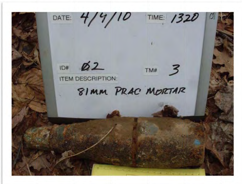
Munitions Debris: 81mm Practice Mortar excavated in SG211
