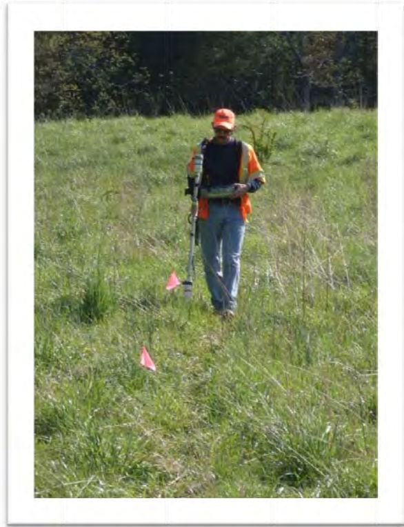
Geophysical Technician collecting data on the Instrument Verification Strip (IVS) with the G-858 Magnetometer in SGL211
