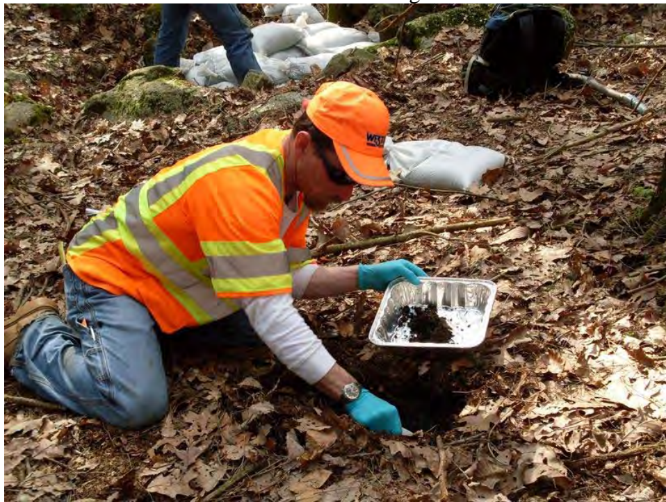
Field Technician taking soil samples in SG211 at detonation location
