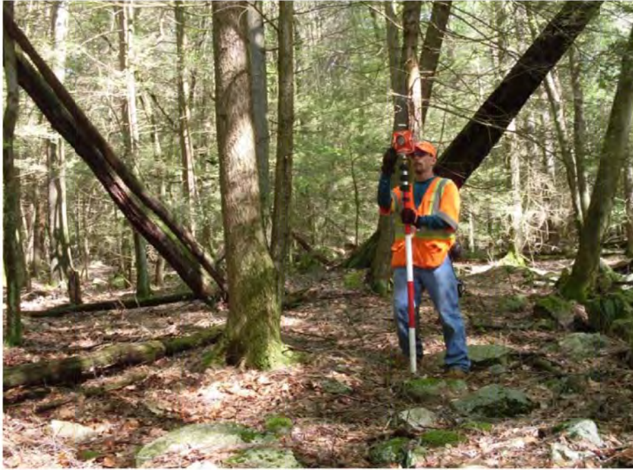
Field Technician establishing survey control in SGL211
