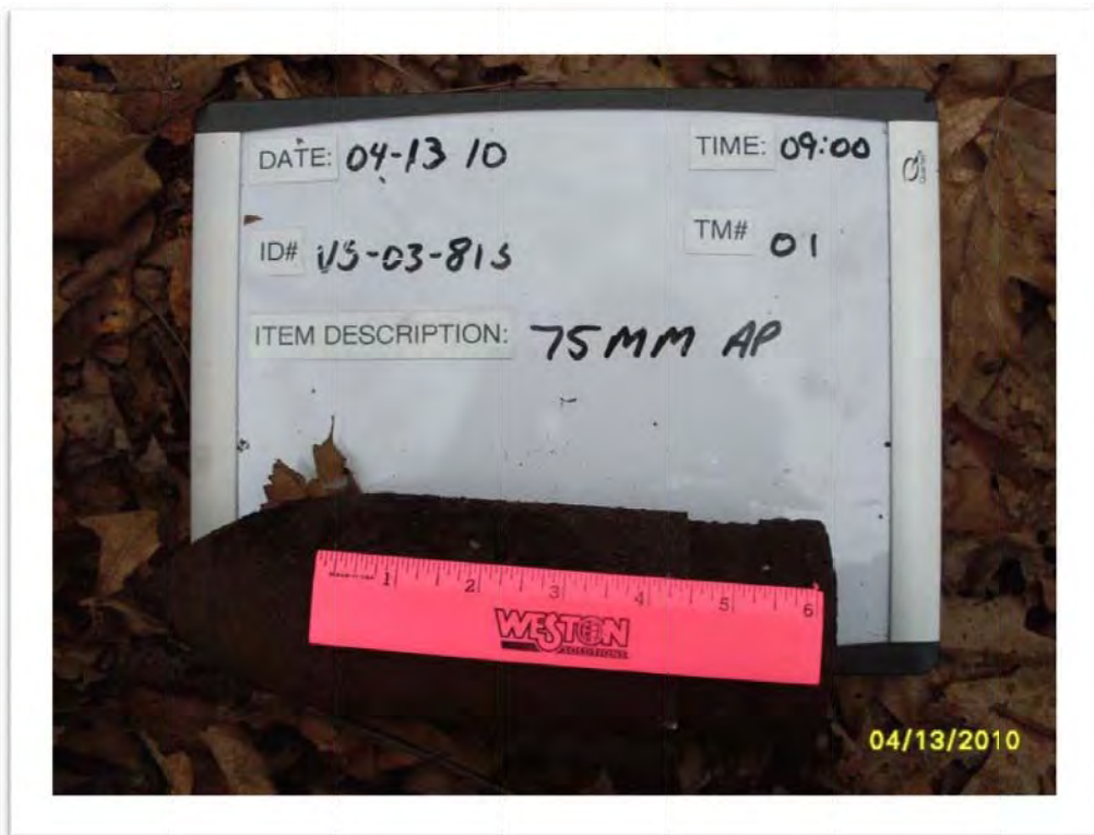
Munitions Debris: 75mm Armor Piercing (solid and inert) excavated in SG211
