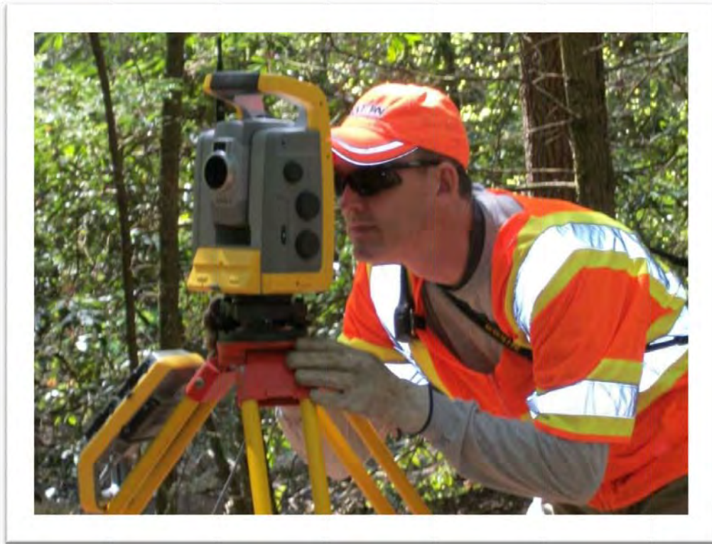
Field Technician calibrating the Robotic Total Station (RTS) for DGM anomaly reacquisition in SGL211
