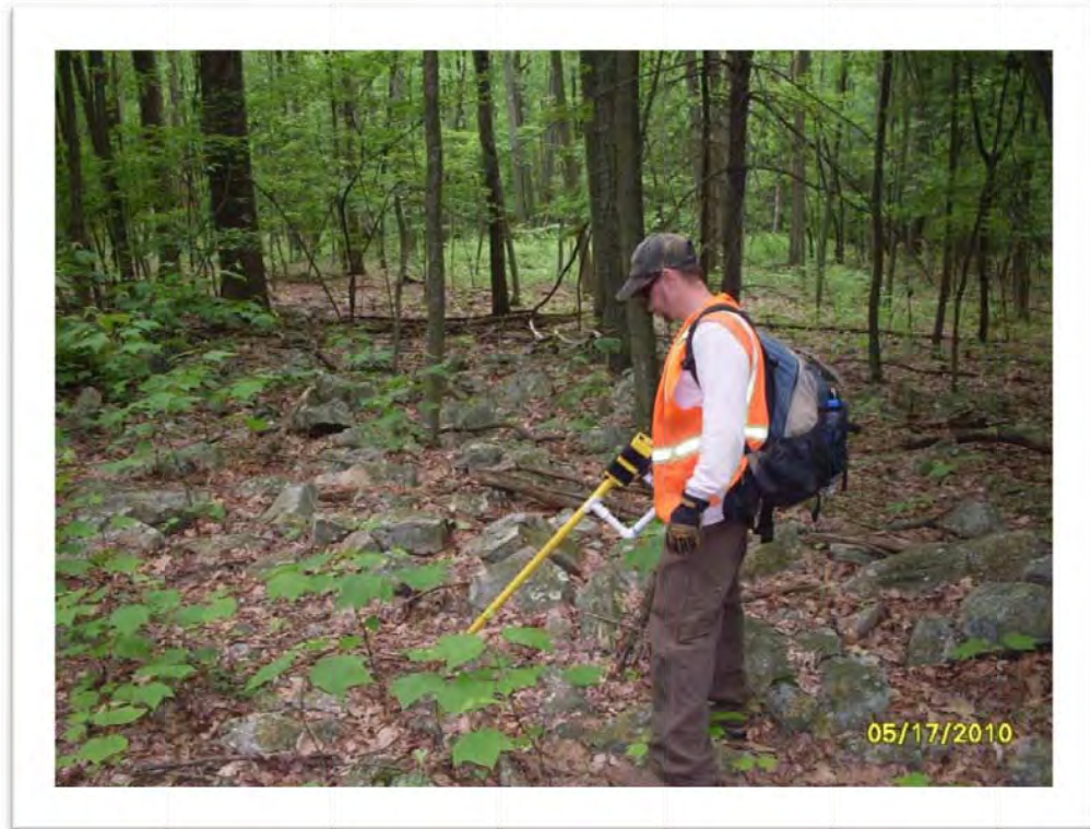
UXO Technician pinpointing an anomaly on an Analog Survey Transect in SGL211
