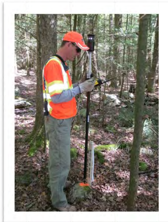
Technician reacquiring DGM anomalies in SGL211
