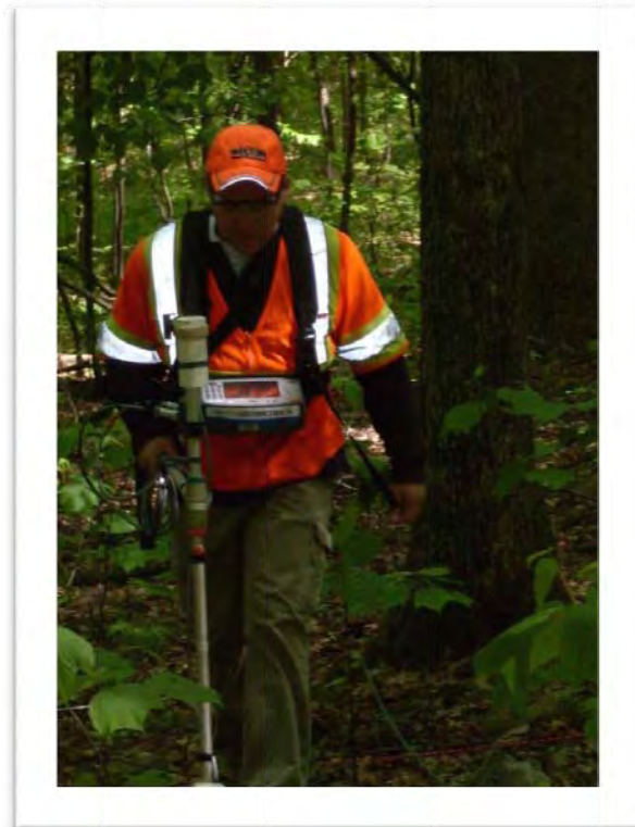
Geophysical Technician collecting data in a DGM grid in SGL211
