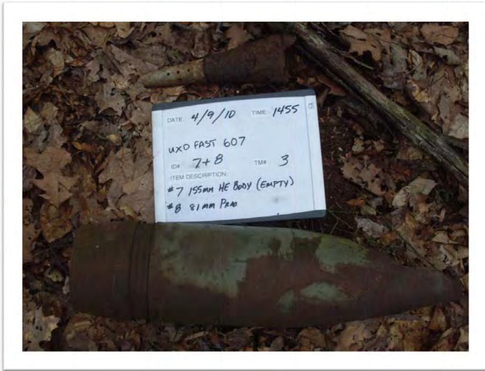
Munitions Debris: 81mm practice mortar and 155mm projectile (empty) excavated in SG211
