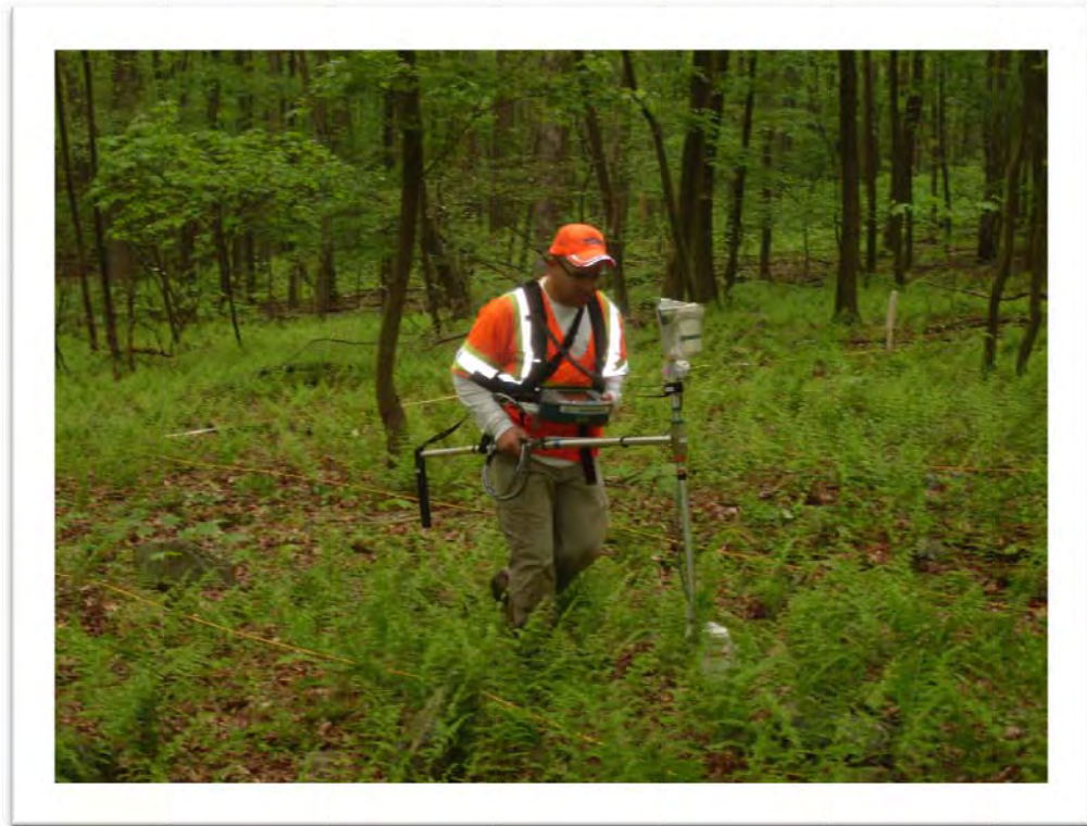
Geophysical Technician surveying a DGM grid with the G-858 magnetometer in SGL211
