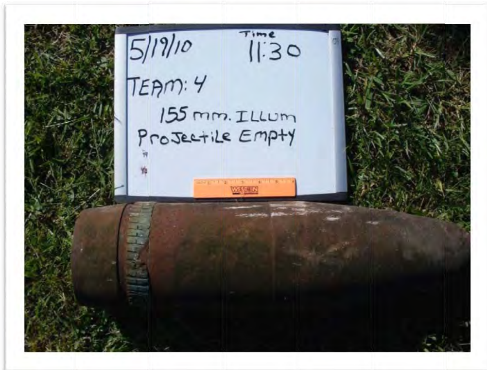
Munitions Debris: 155mm Illumination Projectile (empty) recovered from SGL211.
