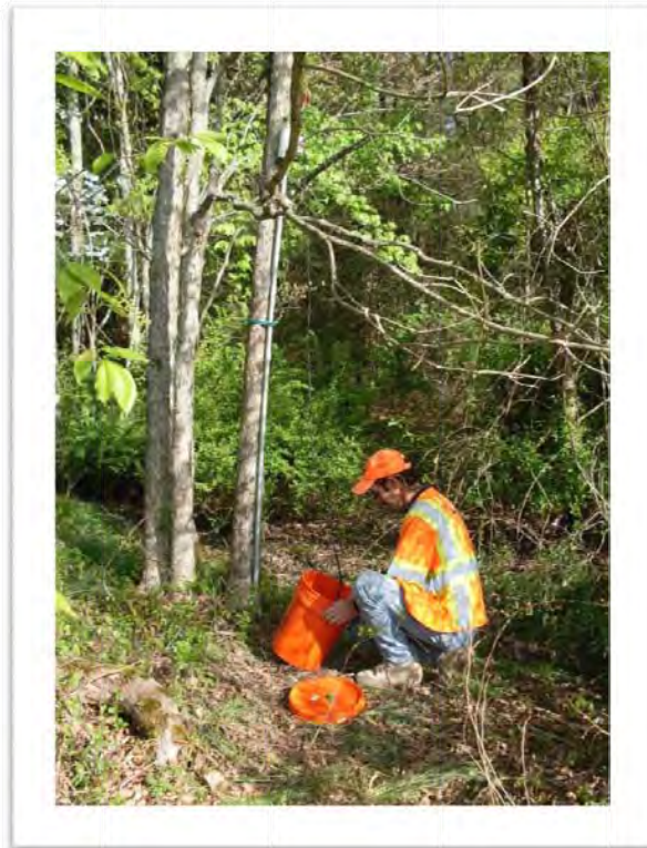
Geophysical Technician setting up the G-856 Magnetometer Base Station in SGL211
