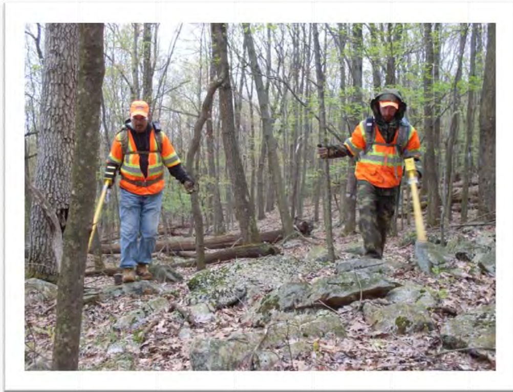
UXO Technicians conducting Analog Assisted Visual Surveys in SG211
