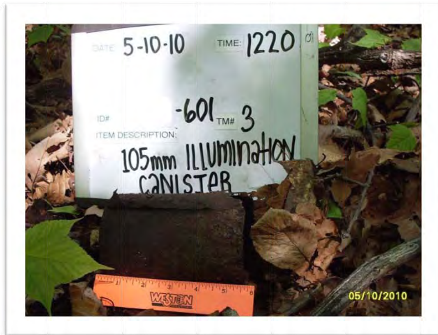
Munition Debris: 105mm Illumination Canister found in SGL211 (see attached map for location).
