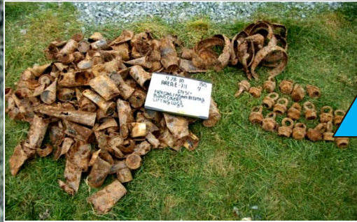
Fuze shipping containers, 155-mm rotating band covers and 155-mm lifting lugs excavated in Area E
