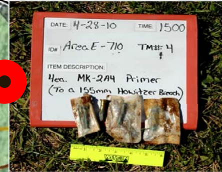
Discarded Military Munitions (DMM) MK-2A4 primers excavated in Area E (1 out of packaging, 3 still in original packaging).
