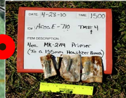
Discarded Military Munitions (DMM) MK-2A4 primers excavated in Area E (1 out of packaging, 3 still in original packaging).
