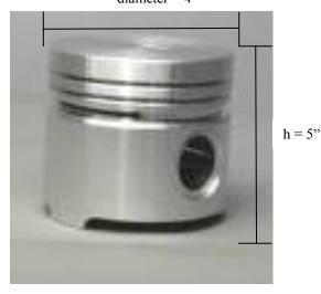
**Example:** What is the surface area of this piston? Radius is  $\frac{1}{2}$  of diameter = 0.5 x 4 = 2" h(height) = 5"
