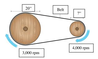
Step 1: Set up the formula for Belt and Pulley Ratio.
