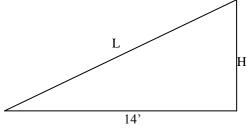
The above sketch is one half of a roof (since most roofs are sloped from the center of the building), with a slope of 6:12.
