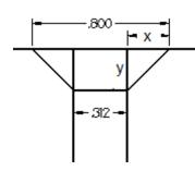
The legs of a 45-45-90 are equal so the depth that the tool needs to be fed (y) is also .244".
