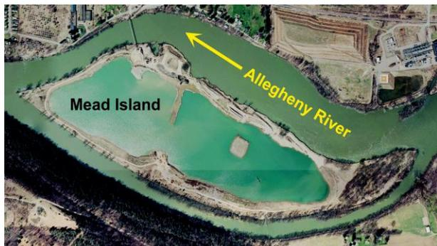
**Figure 7.10.** Allegheny River's Mead Island (RM 184.5-185.6) showing interior pool formed by commercial sand and gravel dredging. Arrow depicts direction of flow (modified aerial photograph from PASDA 2010).
