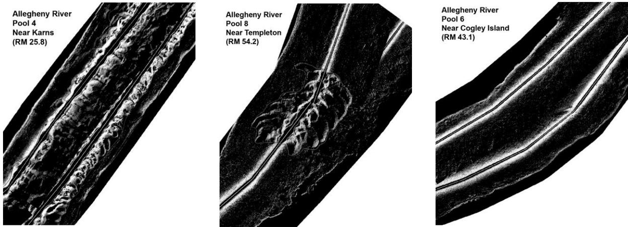
**Figure 6.2.** Side-scan sonar images of extensively dredged reaches of Allegheny River Pool 4 (left); Allegheny River Pool 8 dredge pit with scoop marks from clamshell dredge (center); and for comparison, an undredged reach of Allegheny River Pool 6 (right) (sonar images from USACE 2006).
