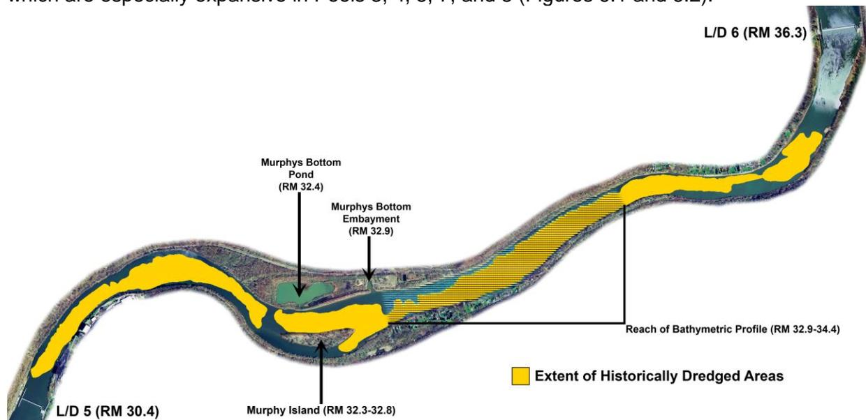
**Figure 6.1.** Dredged Allegheny River Pool 5. Yellow polygons depict historically dredged areas. Cross-hatched area delineates river reach of the bathymetric profile shown in Figure 6.3 (photograph from PASDA 2010; dredged areas from USACE 2006).
