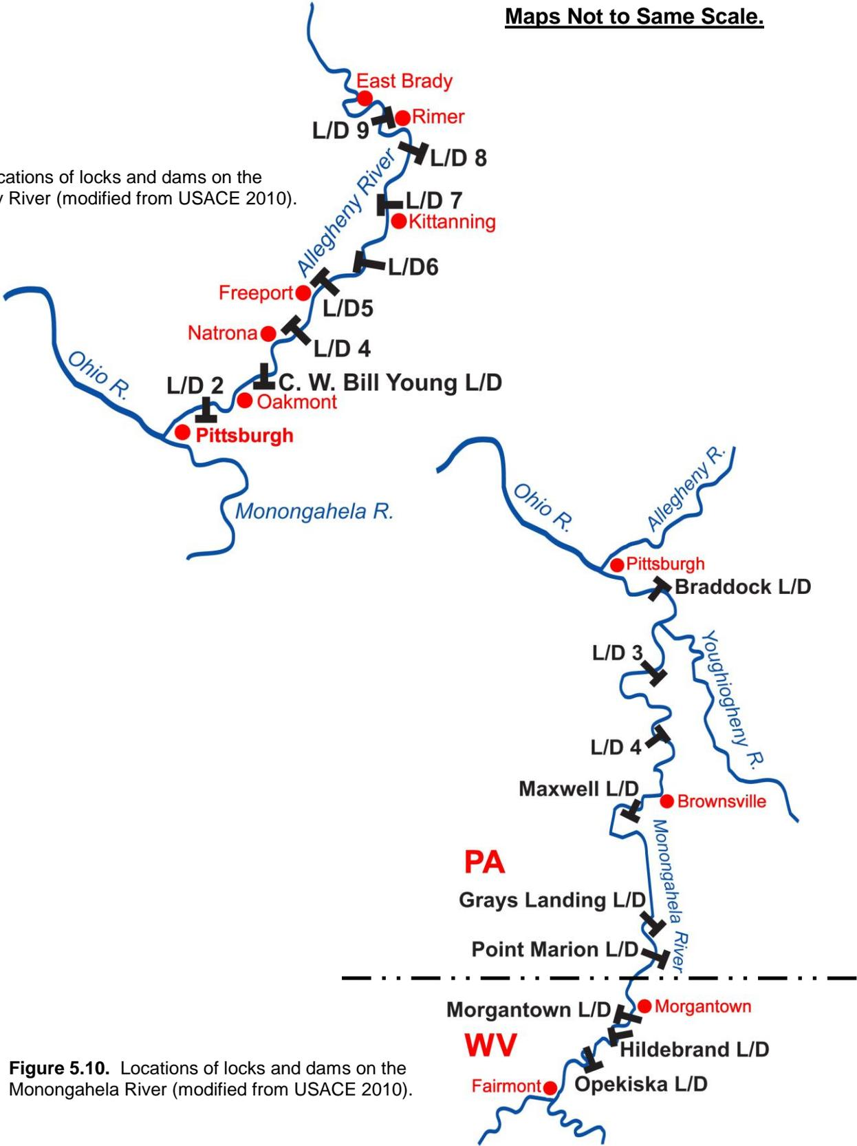
**Figure 5.10.** Locations of locks and dams on the Monongahela River (modified from USACE 2010).
