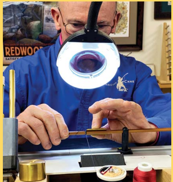
Abbott calls it a wrap packer that he invented and has sold to other rod makers. The small guide squares the thread wrap to the blank and aligns it to the adjacent thread.
