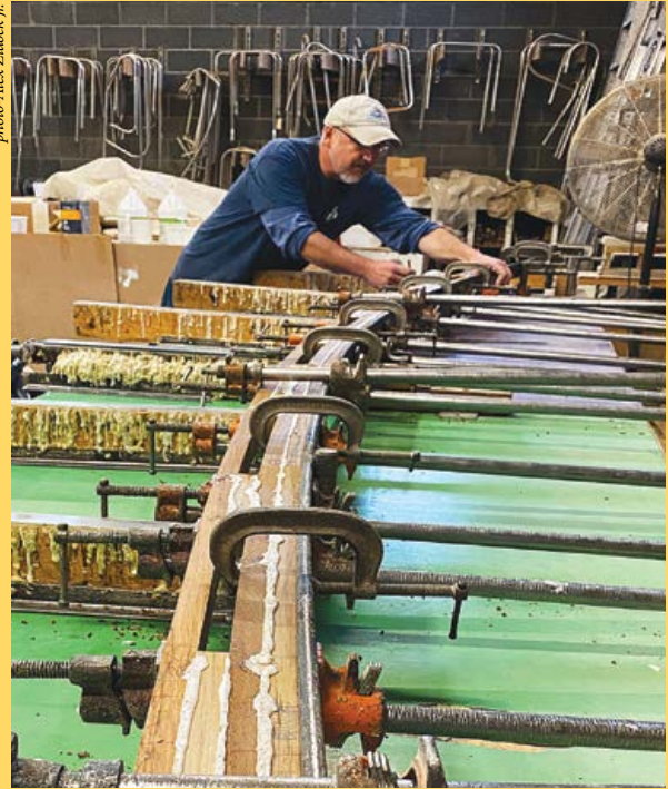
The first teak slats are glued and held in place with 3-inch stainless steel screws. Slats and blocks are put in place until this transom platform, for a 46-foot Grand Banks yacht, reaches 25 inches deep.
