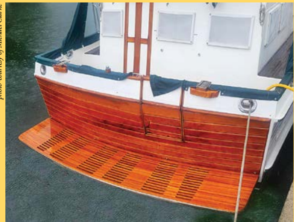
The final teak transom platform built by Butler Marine Products, Luzerne County, matches the original wood of this 46-foot Grand Banks.
