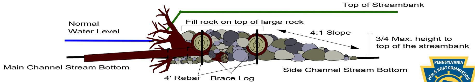
Note: Channel block built lower than surrounding streambanks while maintaining normal water level height
