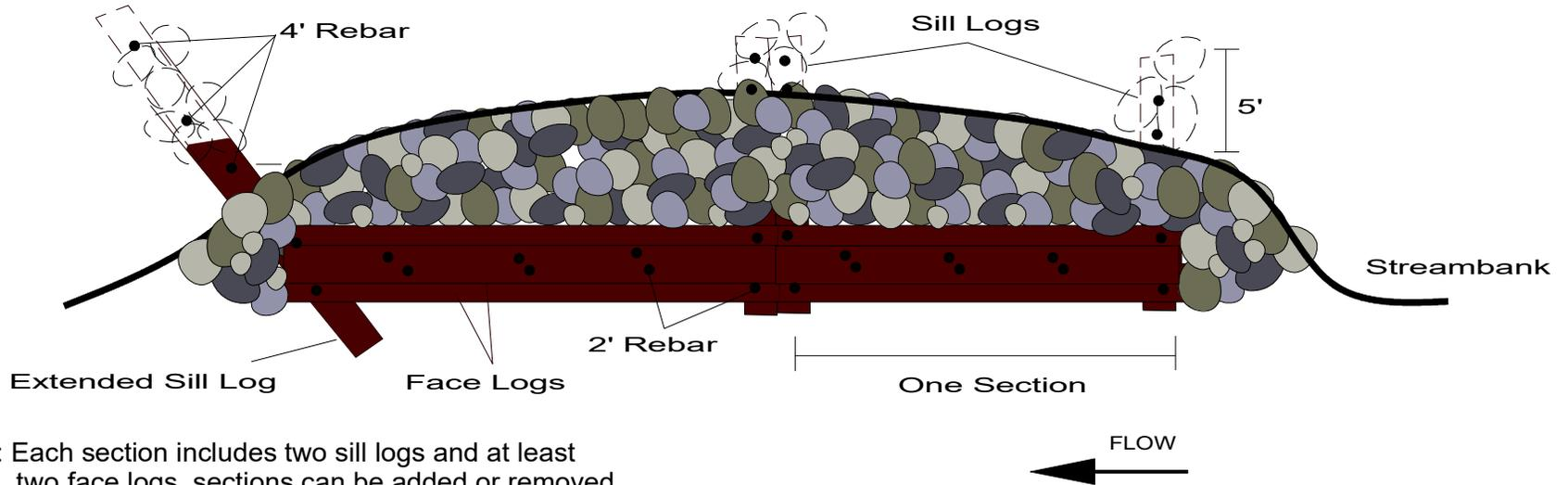
Note: Each section includes two sill logs and at least two face logs, sections can be added or removed
