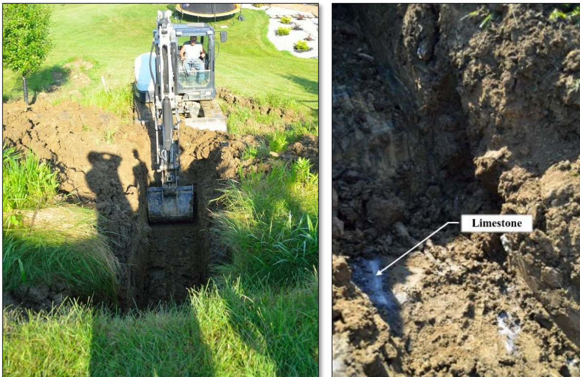
Figure 4-8 - Test pit investigation performed to confirm presence of limestone bed and wet clay soils at toe of slope identified in the desktop study; bag samples were collected for laboratory testing
