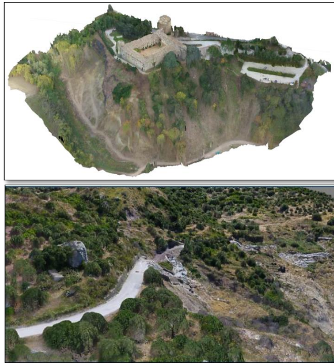
Figure 4-6 - 3D Ortho-Photos projected over the DTM generated from the point cloud [37]
