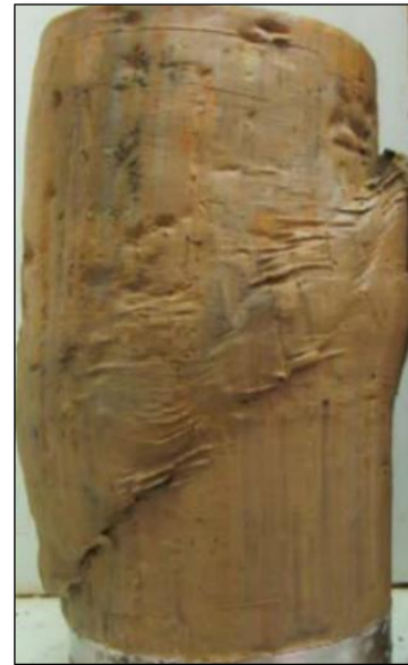
Figure 7-5 - Test Specimen After Consolidated-Undrained Testing
