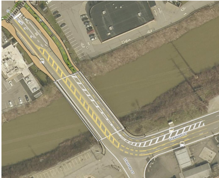
Lane Reduction + Bike Lanes onto Stanhope St
