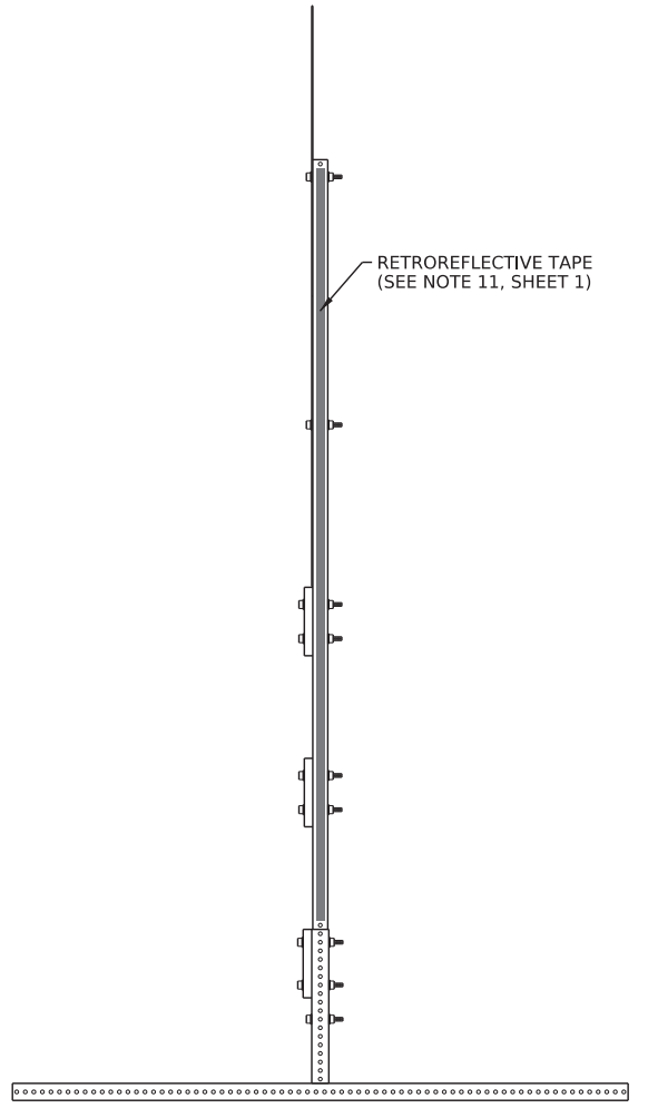
ATTACH TAPE ON LEFT AND RIGHT OUTSIDE EDGE OF POSTS TYPE III BARRICADE RETROREFLECTIVE TAPE REQUIREMENT
