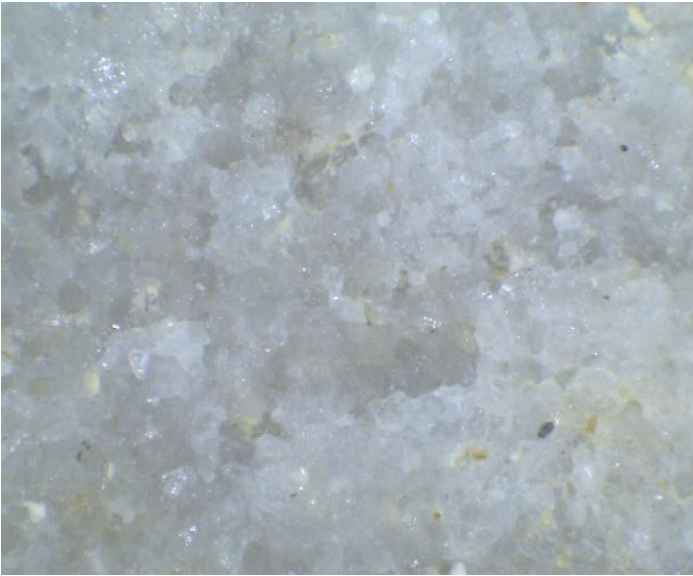
Quartzite at 30x Magnification – Note fusing of grains, low appearance of grain structure, more massive appearance and glassy texture; Other quartzite sample may exhibit a more coarse grained structure, but grains would be fused, with glassy texture and samples would fracture predominantly through grains as opposed to along grain faces.
