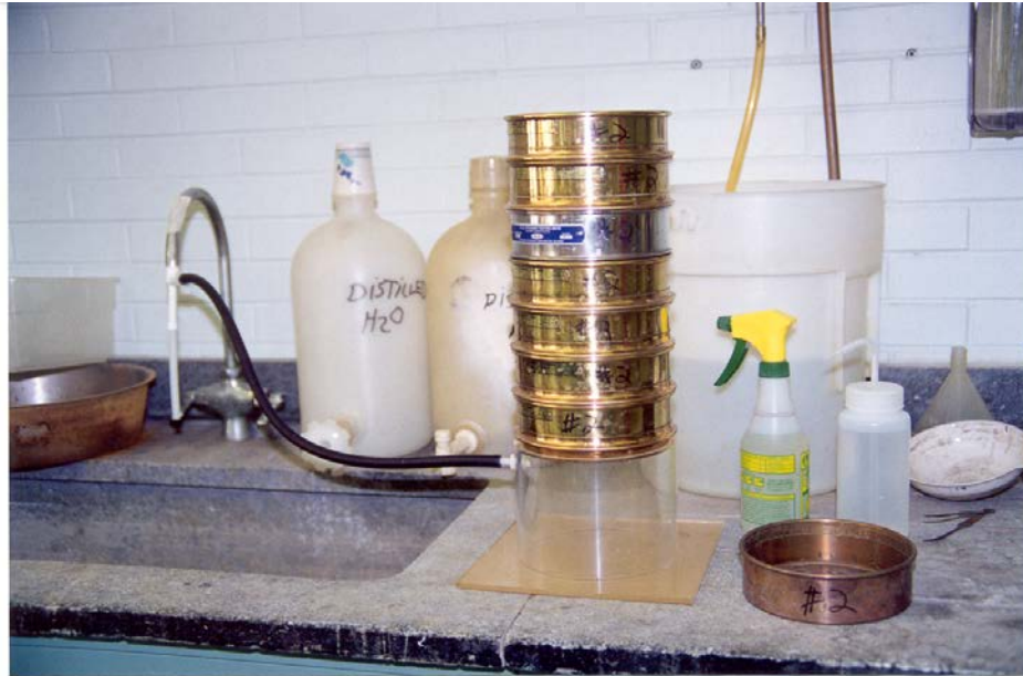
Figure 3- A 152.4 mm (6-inch) sieving cylinder connected to a sink aspirator, with the sieve stack assembled on top of the cylinder.
