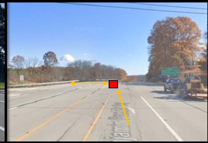
Left turn lanes were shifted to eliminate sight distance conflicts and reduce the amount of time to complete a crossing maneuver
