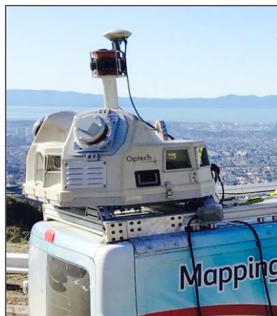
Figure 6. Mobile LiDAR system with spherical camera
