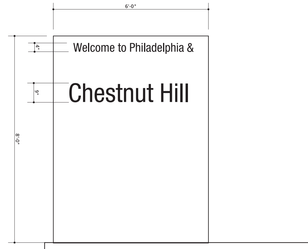
Typical Gateway Sign showing recommended cap height and sign size. Not for design purposes.
